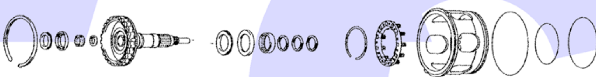
Output Shaft & 'B2' Brake Piston Assembly
