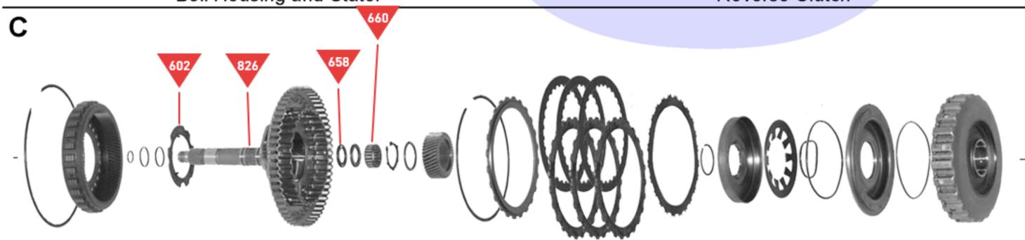
Reverse Planetary, Forward Clutch and Forward Drum
