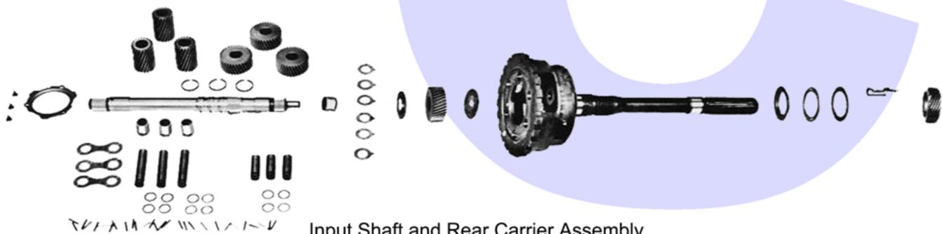
Input Shaft and Rear Carrier Assembly
