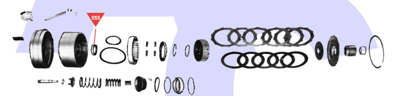
Front Clutch, Servo, Drum and Band
