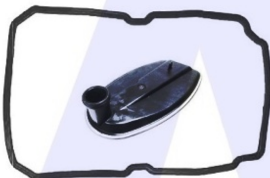
722.6 Pan Gasket M140.GAS01 Filter M140.FIL01
