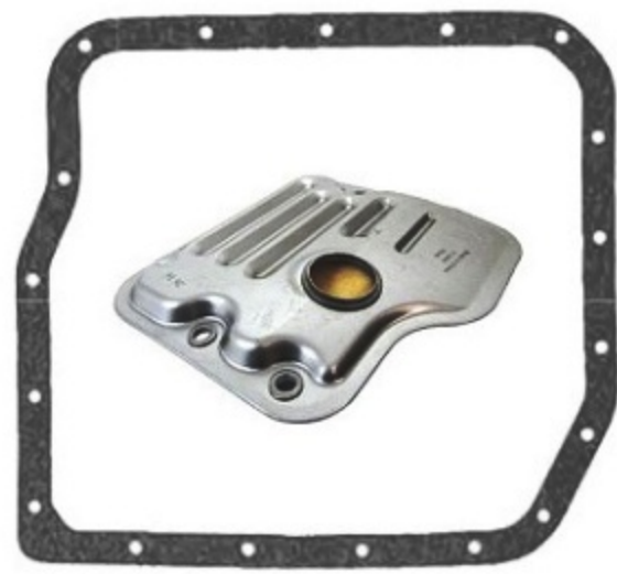
U140E/F, U150E/F, U151E/F Pan Gasket U140.GAS01 Filter U150.FIL01
