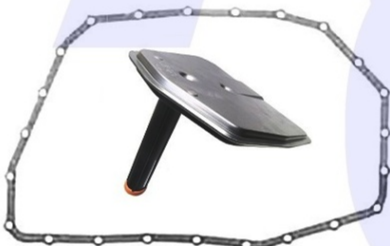
6HP19AV Pan Gasket 6HP19A.GAS01 Filter 6HP19A.FIL01
