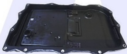
8HP50 / GA8HP50Z Oil Pan & Filter 8HP70.PAN03
